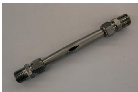
Figure 3.2.3, Burst Test Specimen
