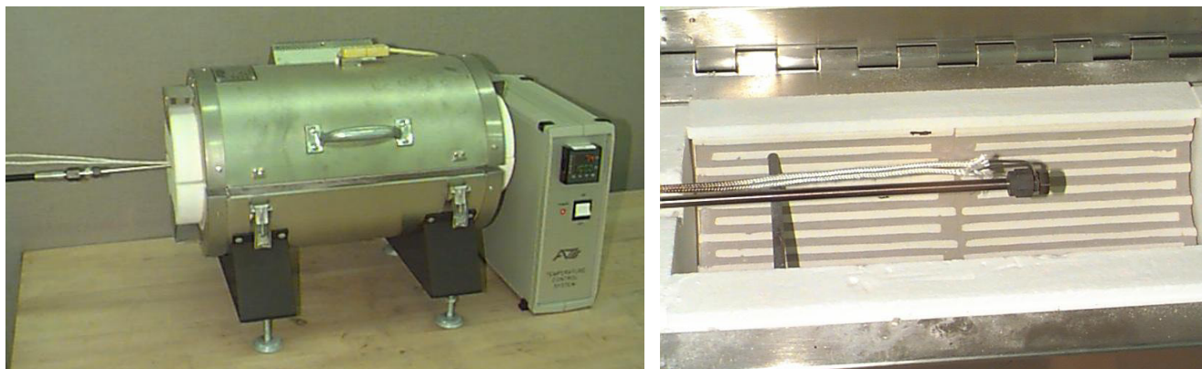
Figure 3.10.1 - 2, Thermal Cycle, Thermal Shock Test Configuration.
