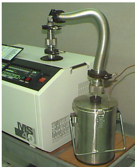
Figure 3.12.1, Low Temperature Helium Leak Test Configuration.
