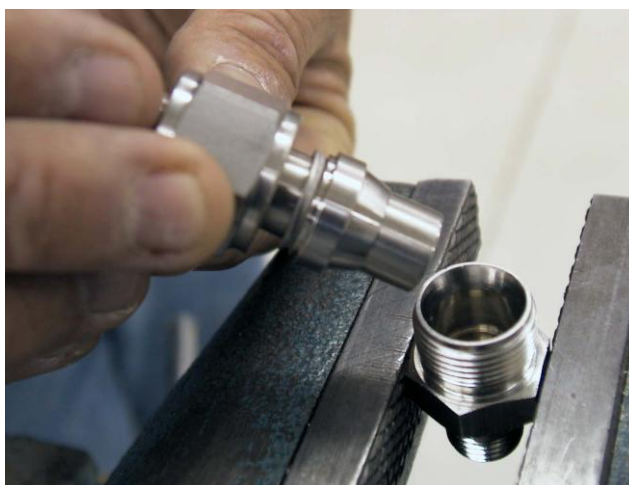
Figure 3.4.1, Repeated Remake Test (Size 8 Griplok)
