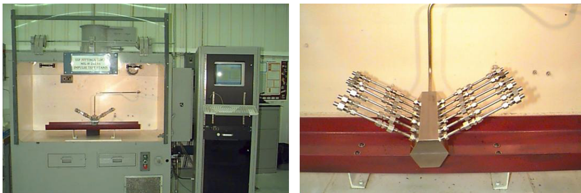
Figure 3.3.1 - 2, Hydraulic Impulse Test Stand and Fixture
