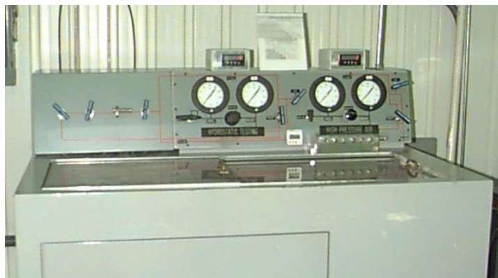
Figure 3.2.1 - 2, Burst Test Configuration
